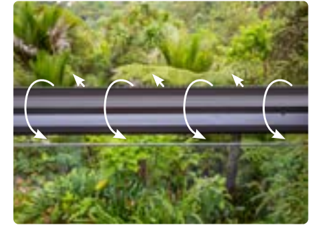
A cat-proof rolling bar attached to a fence prevents cats from getting in and out of the yard.
